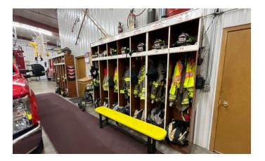
There is also a considerable safety concern for the firefighters who are donning their PPE directly adjacent to the truck floor while there is movement of emergency services vehicles. A safety zone between the truck floor and the turnout area should be provided to keep while firefighters safe preparing for deployment. Wet turn out gear is dried in the apparatus bay using makeshift PVC gear dryers. A floor mounted fan
