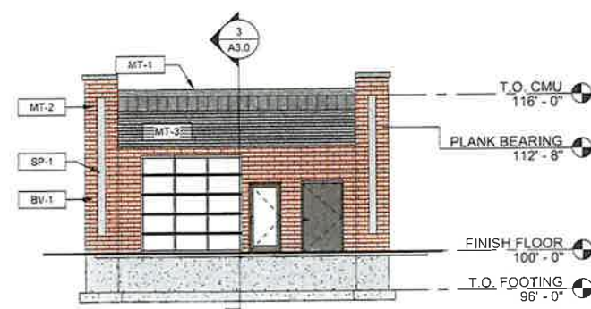
BUILDING ELEVATION - NORTH
