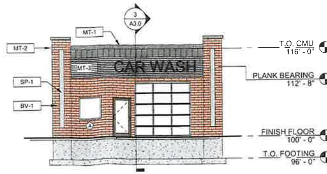
BUILDING ELEVATION - SOUTH
