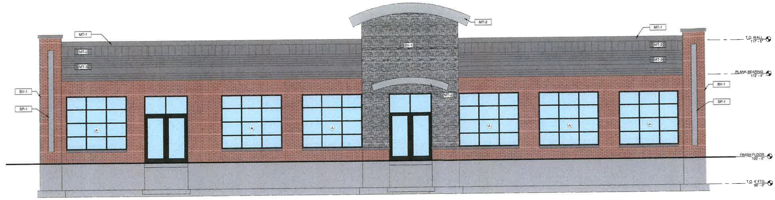
BUILDING ELEVATION - NORTH 1/A2.0 SCALE = 1/4" = 1'-0"
